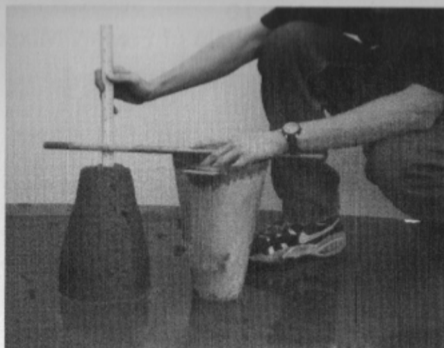
FIGURE A.6 Measuring the slump of freshly mixed concrete.
