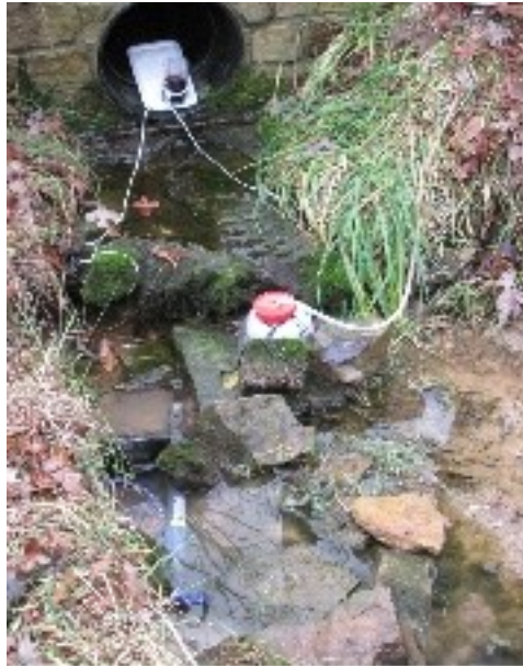
Figure 3.4 Photograph showing the dye and salt release mechanism. Also shown in the picture are the 1 st flush sampler and the YSI datasonde.
