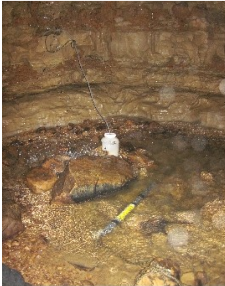
Figure 3.5 Photograph showing the pool at the bottom of Annette's Dome and the beginning of Shaler's Brook. Also pictured is the YSI datasonde (gray and yellow tube in water) and the 1 st flush sampler (white gallon jar).
