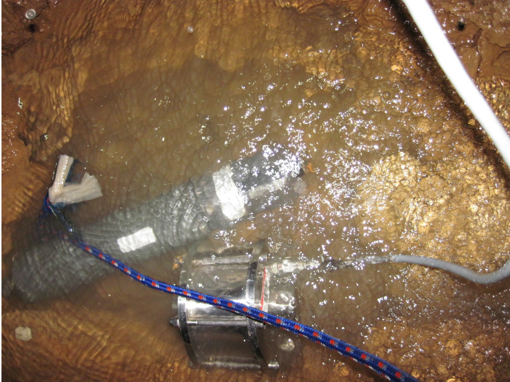
Figure 3.6 Picture showing the GGUN-FL Fluorometer 80526 next to the YSI datasonde in Devil's Cooling Tub on December 20, 2011.
