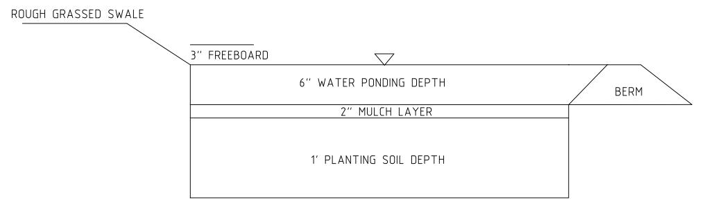
ADPATED FROM A SCHEMATIC IN THE ARTICLE, "BioRetention Cells/Rain Gardens, a Stormwater BMP"
